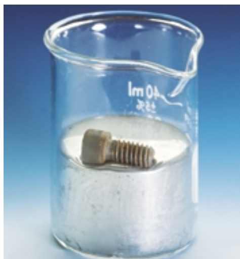
Figure 1.29 Liquid mercury is so dense that it can support a solid iron bolt. A layer of oil has been placed on top of the mercury to prevent vapour from escaping into the surrounding air.
